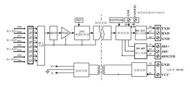
Figure 1 SYAD04A Functional Block Diagram
