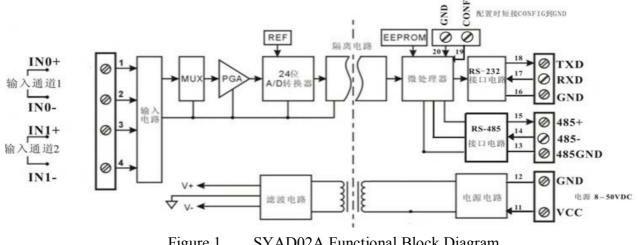
Figure 1 SYAD02A Functional Block Diagram
