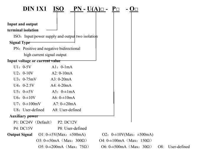
Note: The above voltage output type products need to indicate the output current requirement, and the current output type products need to indicate the load carrying requirement, and the selected value cannot exceed the maximum value (Max).
